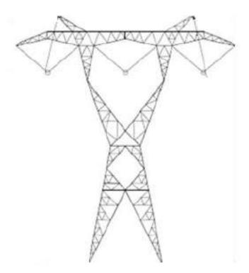
Figure A-3: Tower Type 515 (Self Support).
